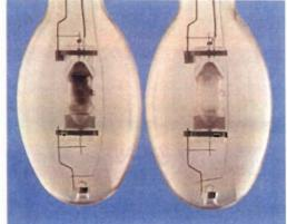
Unaltered photo of two 400W typical lamps, taken at mean lamp life (8,000 hours). Note the difference in arc tube condition. The lamp on the left shows the arc tube blackening effect caused by the use of magnetic ballasts. The lamp at the right shows the minimal arc tube discoloration that is characteristic of lamps operated on an electronic ballast The lamp on the right is capable of generating at least 15% more mean lumens than the magnetically ballasted lamp at the left.
